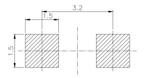
**Note:** Tolerances Unless Dimension is  $\pm 0.1$ mm, Unit = mm
